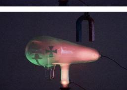
☐ High voltage applied across electrodes ionize the gas forming plasma. Accelerated electrons of the plasma do not reach the screen due to the obstacle placed in-between and so cast a shadow. When a magnet brought near the plasma the electron beam bends and so the shadow is
